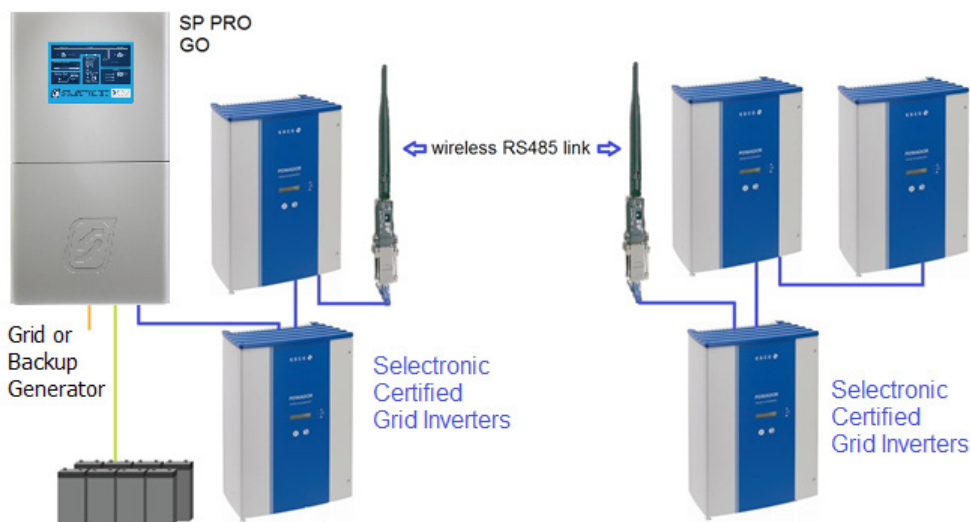
RS485 wired AND wireless communications links between SP PRO GO and Selectronic Certified inverters
