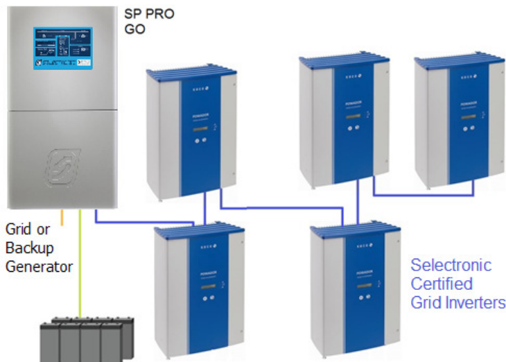
RS485 wired communications links between SP PRO GO and Selectronic Certified inverters
